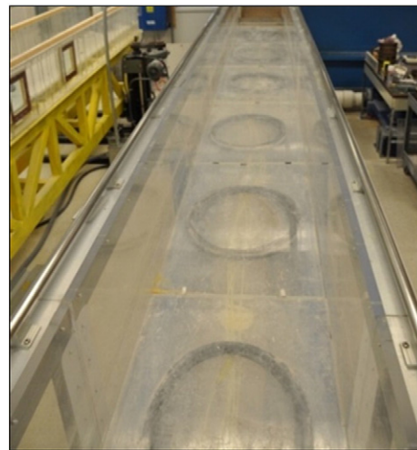
Fig. 1. Bedload monitoring system without sediment. View is looking down the flume. The Plexiglas plates and pressure tubes underneath are visible. The latex sheet and sediment have not yet been added.
