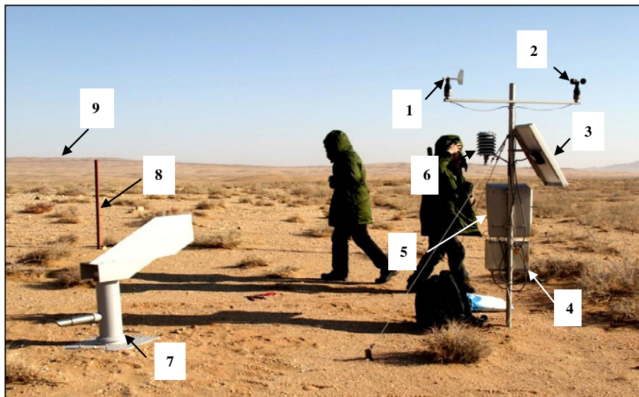
Fig. 2. Instruments used to measure meteorological data. 1. Wind vane. 2. Propeller anemometer. 3. Solar panels. 4. Battery. 5. Datalogger. 6. Temperature and humidity sensor. 7. Sediment collector. 8. Fence. 9. Shifting dune. The picture was from Yang et al. (2014).
