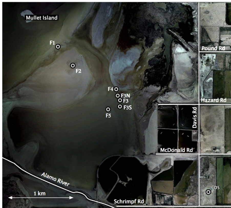
Fig. 2. Annotated Google Earth image of the fumaroles in our study area from Table 1. Mullet Island is upper left, the Davis–Schrimpf gryphons at lower right (DS). The evident NW-trending lineament of the geothermal features is suggestive of a fault, probably the Calipatria Fault (Lynch and Hudnut, 2008).
