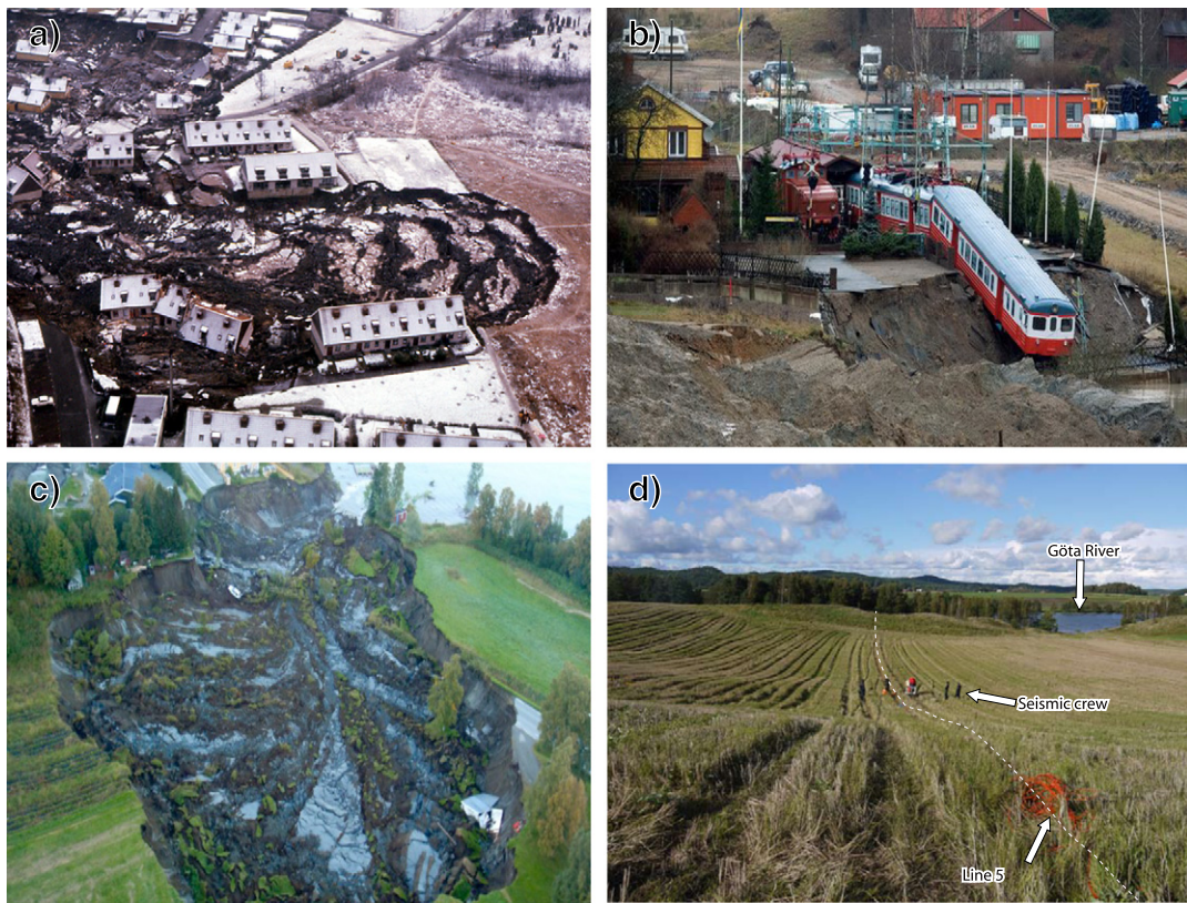
Fig. 1. Example figures showing major quick-clay landslides and their impacts. (a) Tuve landslide, Sweden in 1977 and (b) Småröd landslide, Sweden in 2006 (courtesy of the Swedish Accident Investigation Authority, SHK). (c) Lyngseidet landslide, Norway in 2010; it was likely triggered by loading of materials next to the shoreline (courtesy of the Geological Survey of Norway, NGU, photo: Andrea Taurisano, NVE). (d) Fråstad landslide in our study area next to the Göta River (photo by Alireza Malehmīr, 2011).
