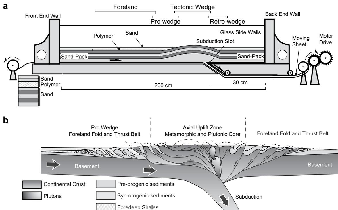
Fig. 1. (a) Apparatus design used in these Experiments, and (b) comparison with model for a doubly vergent wedge (modified from McClay and Whitehouse, 2004).
