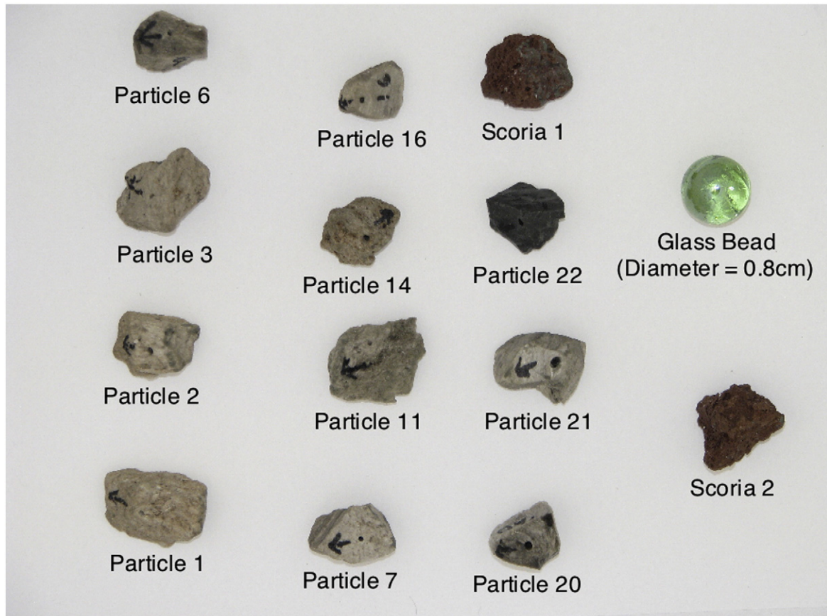
Fig. 1. Particles for which we measured heat transfer coefficients. Properties are listed in Table 1. In some particles, the hole into which the thermocouple was placed can be seen.
