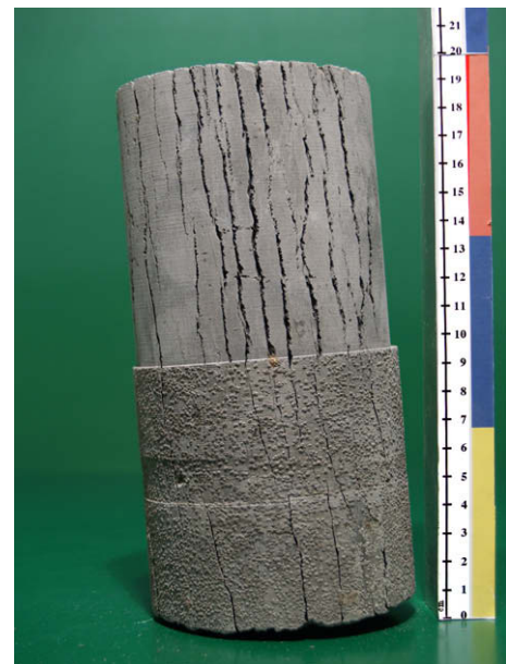
Fig. 1.2. Ageing cracks in plastic bag sealed sample.
