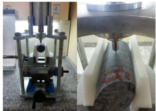
Fig. 2. Cerchar apparatus and sample.
