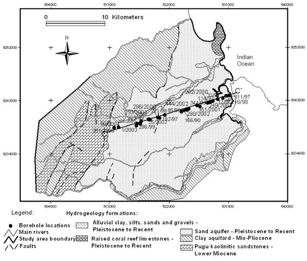
Fig. 1. Hydrogeological map of the study area with location of boreholes used in the cross section.
