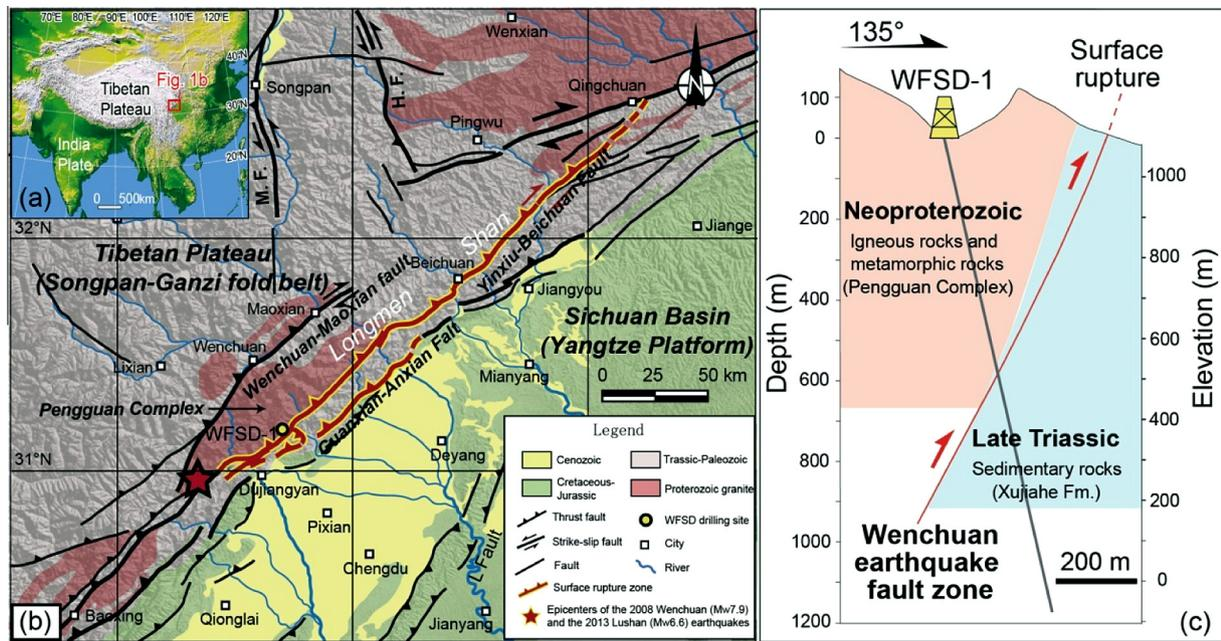
Fig. 1. Simplified geologic and active tectonic map of the Longmen Shan and its adjacent area (modified from Li et al., 2014). (a) Location of the study area. (b) Geological map of Longmen Shan around the WFSD-1 drilling site. (c) Simplified geologic cross-section at the WFSD-1 drilling site.
