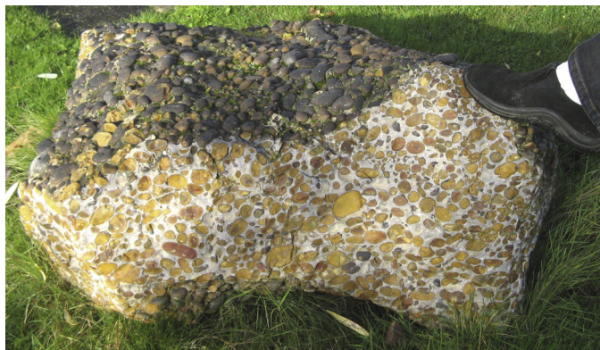
Fig. 2. A puddingstone from the Colliers End outlier with very well rounded, internally stained pebbles in a fine pale matrix. The rock is cohesive and fractures evenly across pebbles and matrix. Grey and brown coated pebbles stand out on the edges of the concretions where the cement ends.
