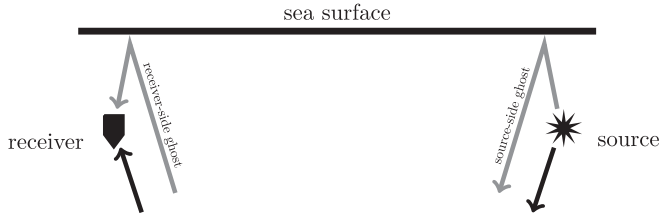
Fig. 1. Graphical representation of source-receiver configuration with source-side and receiver-side ghosts.
