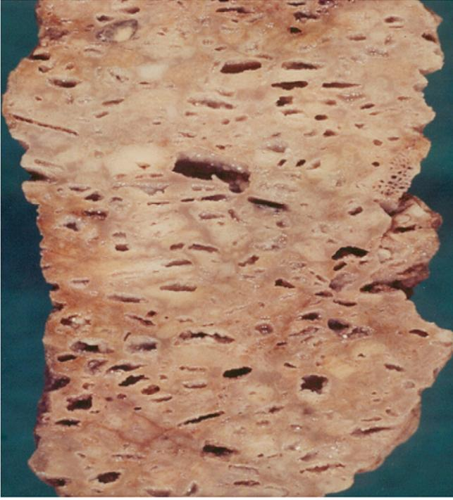
Fig. 1. Example of a double-porosity carbonate rock.
