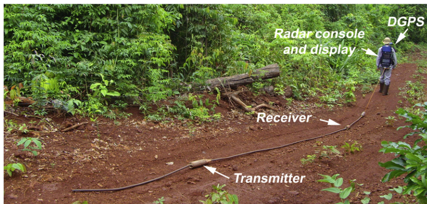
Fig. 1. 40 MHz towed GPR system with collinear antennas housed in flexible hose. The backpack contains a radar control unit and a DGPS receiver as well as the radar display.
