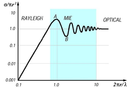
Fig. 1. Scattering cross-section as a function of the object dimension normalized ( $2\pi \cdot r$ ) by the geometric cross-section ( $\pi r^2$ ) and the signal wavelength ( $\lambda$ ), respectively. The sphere of arbitrary dimension is a perfectly conducting and excited for a single frequency signal (Skolnik, 1970).
