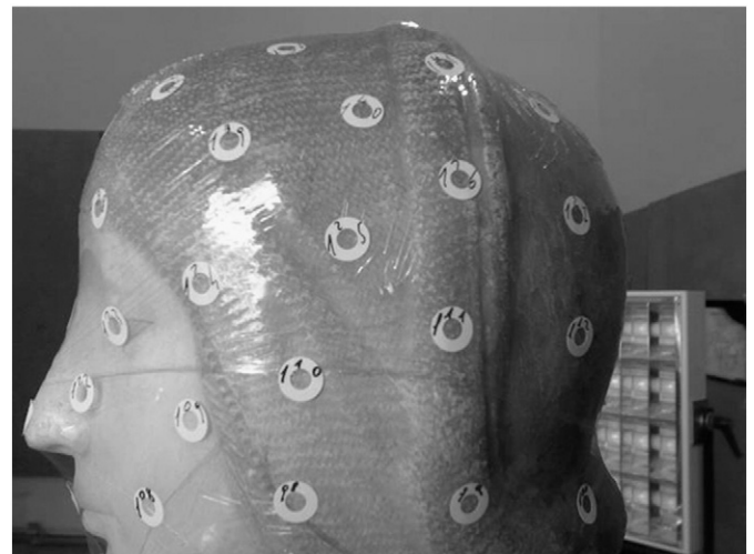
Fig. 2. Measurement points were placed on a transparent film used to avoid damages on the surface.
