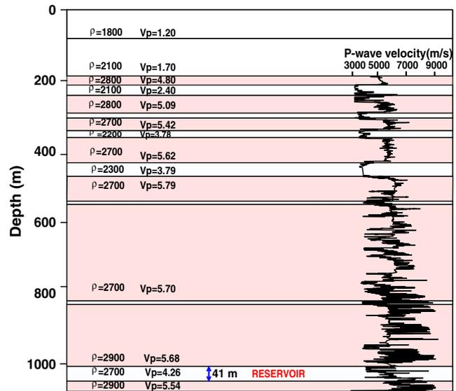
Fig. 2. Schematic diagram of multi-layered geological model. Units of density and velocity are in kg/m<sup>3</sup>, km/s, respectively. The model parameters are estimated by averaging layers from the sonic log shown.
