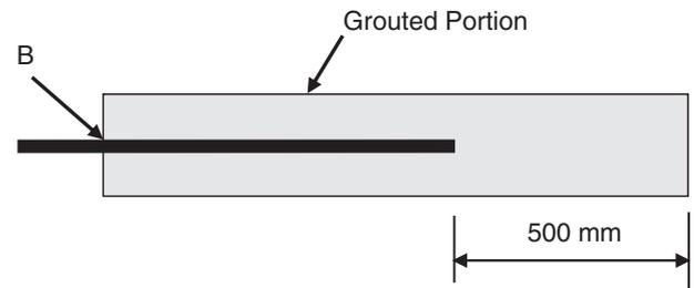
Fig. 2. Rock bolt with insufficient rebar length.
