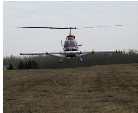
Fig. 3. Bell 206L model helicopter collecting magnetometer data at Yekau Lake, Canada
