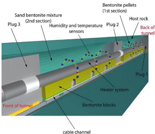
Fig. 1. Lay-out of the HE-E experiment (Teodori and Gaus, 2011).
