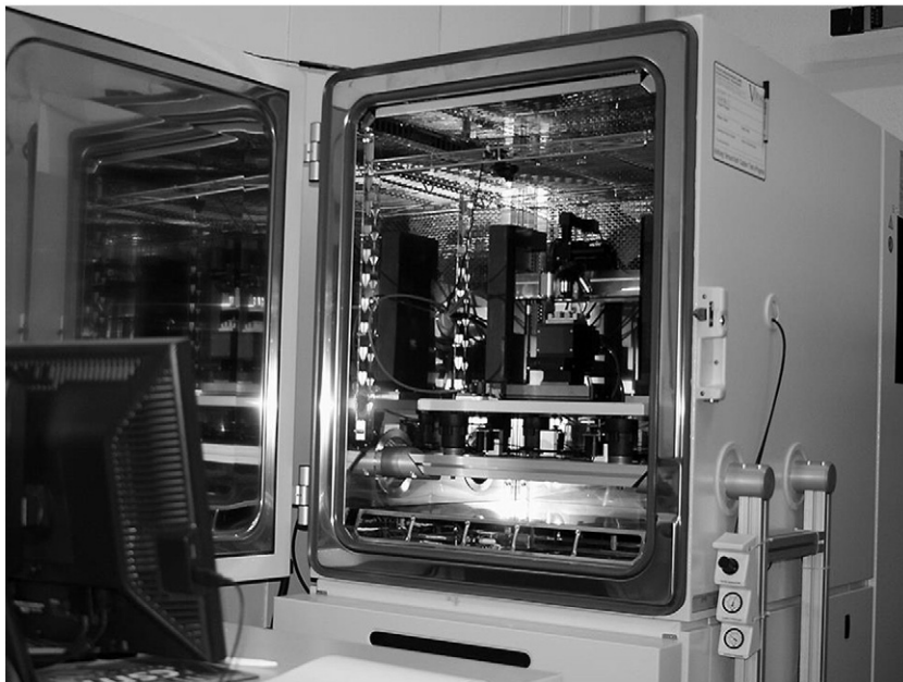
Fig. 1. Nano-indentation tester installed in climatic chamber.
