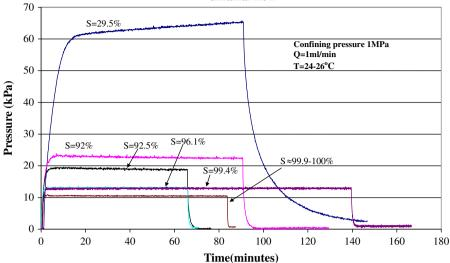
Fig. 1. Influence of the degree of saturation on the development of steady state pressure-one-dimensional pressure test (Selvadurai, 2009).
