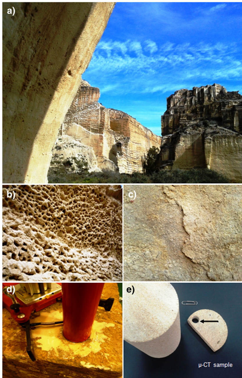
Fig. 1. a. General view of the quarries; b. Alveolization ; c. Sanding and peeling deterioration; d. Drilling machine extracting cylindrical cores to carry out physical tests; e. Subsample used in the micro-CT measurements.
