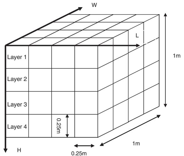
Fig. 3. Schematic diagram for sampling a one-meter cube.
