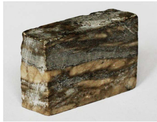
Fig. 1. Rectangular ( 37 \times 23 \times 11 mm) rock block, taken from a Gipskeuper horizon in an aquifer near the Birs river in Switzerland (Epting et al., 2009a,b). The white parts are few millimeters wide and are the only soluble (gypsum) parts of this sample.
