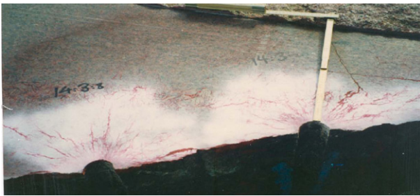
Fig. 2. Radial cracks observed around ( \varnothing 64 mm blast-holes from a bench blast and 0.5 m by 0.5 m burden and spacing respectively). The explosive used was Kumulux with 22 mm cylindrical column charge, with the holes blasted instantaneously (Olsson and Bergqvist, 1995).
