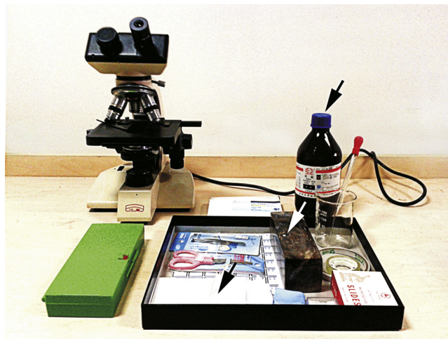
Fig. 2. The fossil wood and parts of the experiment equipment and reagents. The upper black arrow indicates acetone; the middle white arrow shows the polished fossil wood, collected from one of the handicraft shops in Chaoyang; registration number: PMOL-B01396; the lower black arrow indicates white cellulose acetate sheet named “Cellulose acetate layer sheet” with the product number 68003461.
