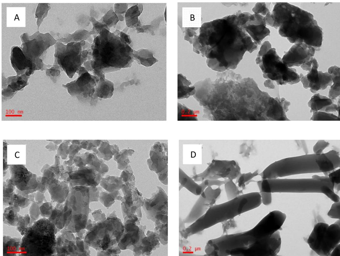
Fig. 1. TEM images of Cu-MOF samples: (A) Cu-BTC-1, (B) Cu-BTC-2, (C) Cu(tpa) and (D) Cu(im)<sub>2</sub>.
