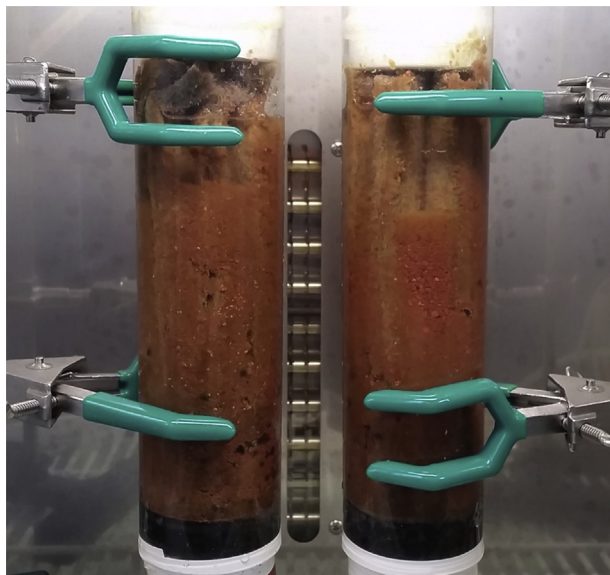
FIG. 1. Configurations of up-flow reactor packed with nonwoven fabric material in a thermostatic incubator set to 20°C: Low-R1 (left) and Low-R2 (right) on day 949. The nitrogen removal performance of both reactors was 1.5 kg-N/m 3 /day as NRR with 1.7 kg-N/m 3 /day as NLR.
