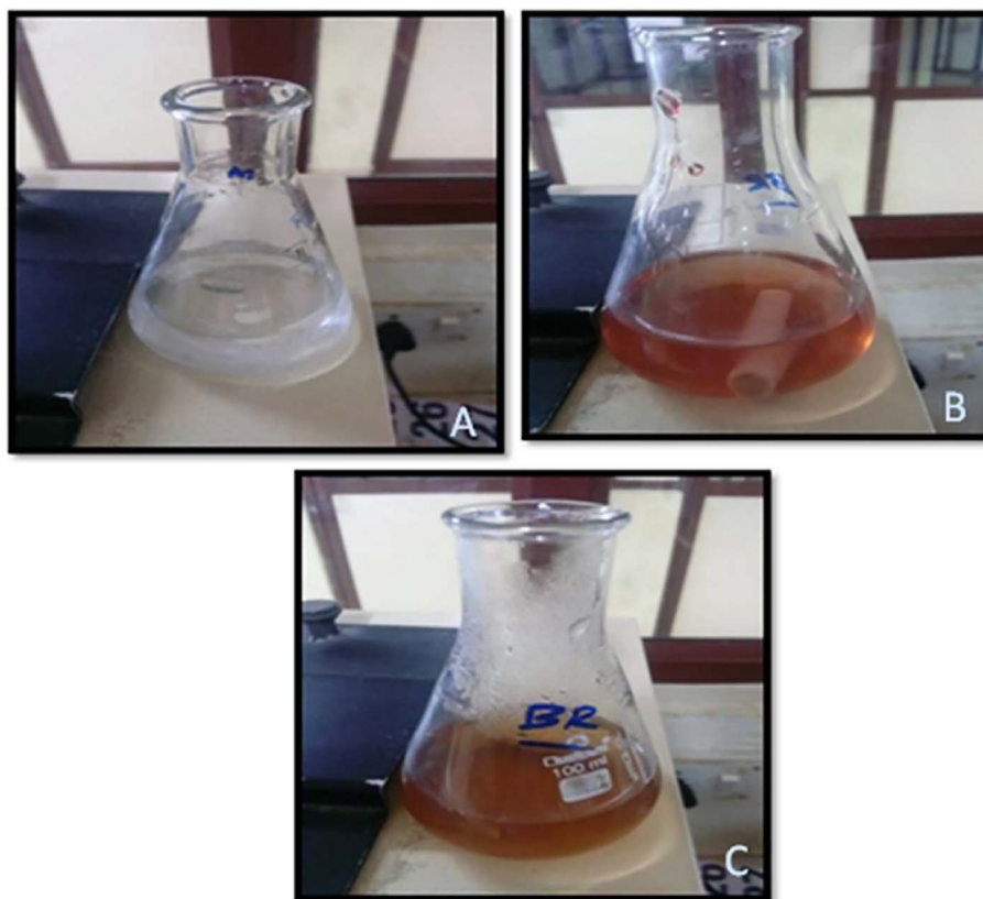
Fig. 1. Nanoparticle synthesis using Beta vulgaris plant extract; (A) Silver nitrate solution, (B) Beta vulgaris extract broth, (C) Silver nanoparticle solution.
