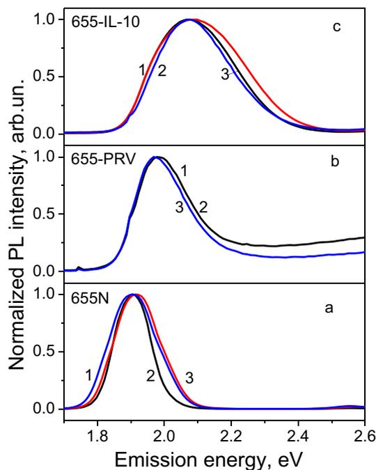
Fig. 2. PL spectra of three non-conjugated 655N (a) and three bio-conjugated 655-PRV (b) and 655-IL-10 (c) QD ensembles.
