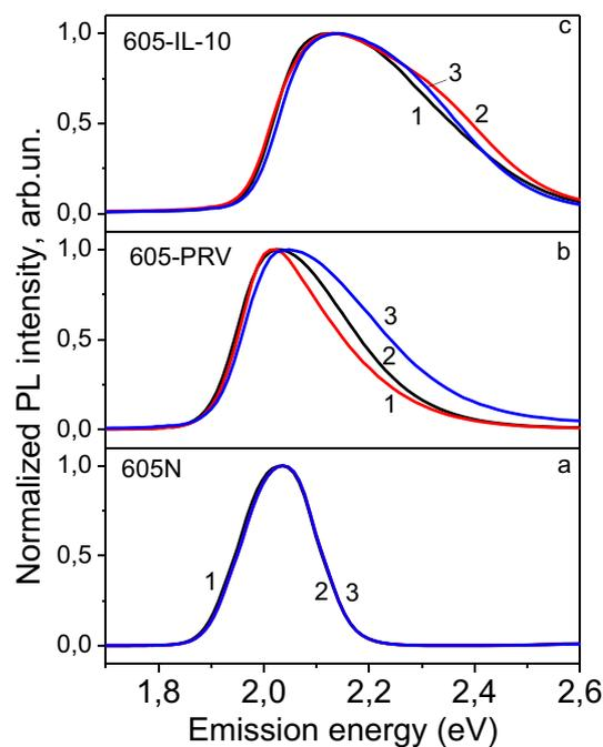
Fig. 1. PL spectra of three non-conjugated 605N (a) and three bio-conjugated 605-PRV (b) and 605-IL-10 (c) QD ensembles.
