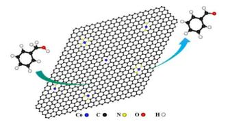
Atomically cobalt dispersed onto nitrogen-doped graphene has extremely high atom efficiency and shows high activity for the selective oxidation of alcohols by oxygen molecule.
