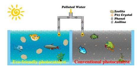
Eco-friendly photocatalyst is developed by fixing classic photocatalysts into zeolite crystals to impart shape-selective catalysis for the pollutants removal but eco-friendly for organisms.
