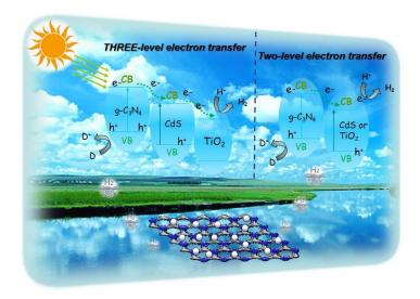
Carbon nitride coupled with CdS- $TiO_2$  nanodots as 2D/0D ternary composite with enhanced photocatalytic  $H_2$  evolution: A novel efficient three-level electron transfer process
