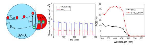
The combination of  $BiVO_4$  photoanode and an ultrathin  $Fe_2O_3$  film as cocatalyst, which will cause upward-bent band in  $BiVO_4$  faciliating the holes transfer, can greatly improve the photocurrent density and IPCE of  $BiVO_4$  photoanode.
