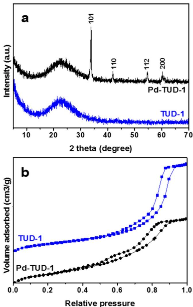
Fig. 1. a) The XRD patterns of Pd-TUD-1 and the neat TUD-1 materials, b)  $\text{N}_2$  physiosorption isotherms of Pd-TUD-1 and TUD-1.
