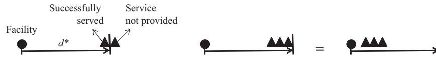
Fig. 1. Two examples where a binary coverage function may not be an appropriate choice for coverage definition. Left: two adjacent demand points are arbitrarily labeled as success vs. failure. Right: advantage (better service quality) provided by a server on the right is not accounted for.
