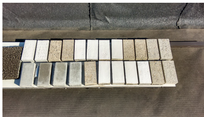
Fig. 1. Natural ageing on the roof top of the BRRC building in Sterrebeek (Belgium).
