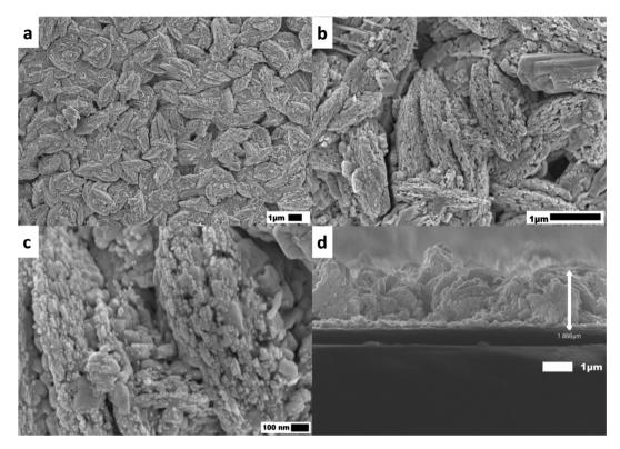
Fig. 1. Low-resolution (a) and high-resolution (b, c) top view SEM images of CuWO<sub>4</sub> on FTO surface annealed at 500 °C. (d) Cross-sectional SEM image of CuWO<sub>4</sub> on FTO.
