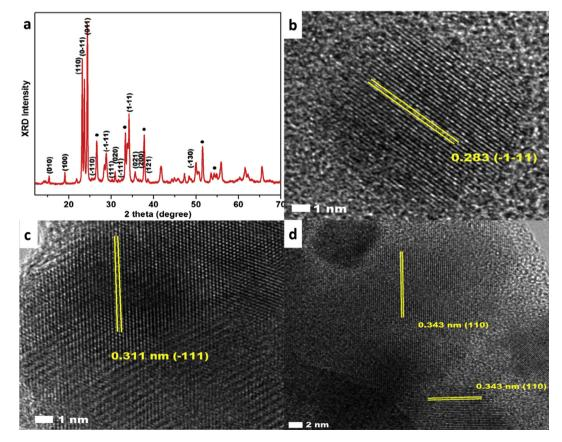
Fig. 2. (a) XRD patterns of CuWO<sub>4</sub> annealed at 500 °C for 2 h. (b-d) shows typical HRTEM images with corresponding *d*-spacings of CuWO<sub>4</sub>.
