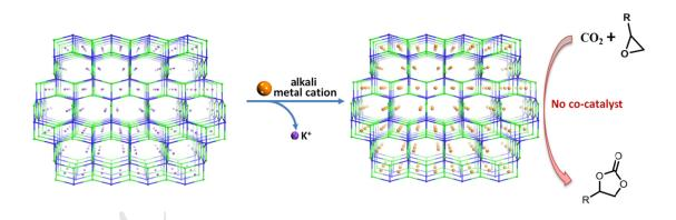
A series of M-UTSA-16 (M = Li, Na, K, Rb, Cs) possessing analogous structures with various alkali metals by cation-exchanged method exhibited efficiently catalytic performance for cycloaddition reaction from  $CO_2$  and epoxides in the absence of cocatalyst.
