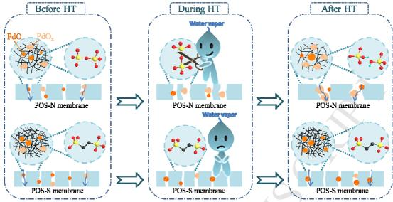
As the content of SiO $_{4/2}$  in the POS-S membrane is very low, so Si-O-Si groups are not displayed to simplify the schematic diagram. III = hydrothermal treatment; PdO $_x$  = intermediate Pd oxide
