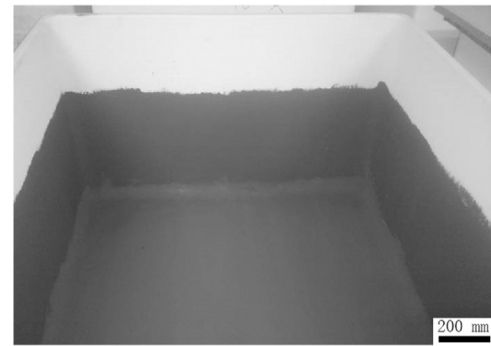
Fig. 1. Optical image of the crucible with silicon powder coating for ingot B.
