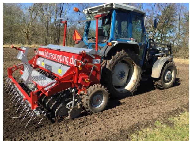
Fig. 1. Experimental seed drill from Kongskilde modified with the coulter depth measurement system.
