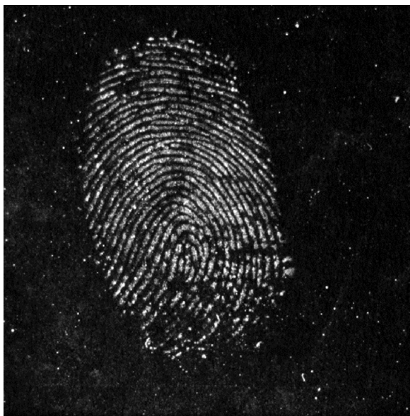
Fig. 1. A latent fingerprint on a polymer banknote that has been treated with fpNatural 1™ fingerprint powder and visualised under 600–650 nm illumination with 715 nm long-pass camera filter using a Foster + Freeman Crime-lite Imager.
