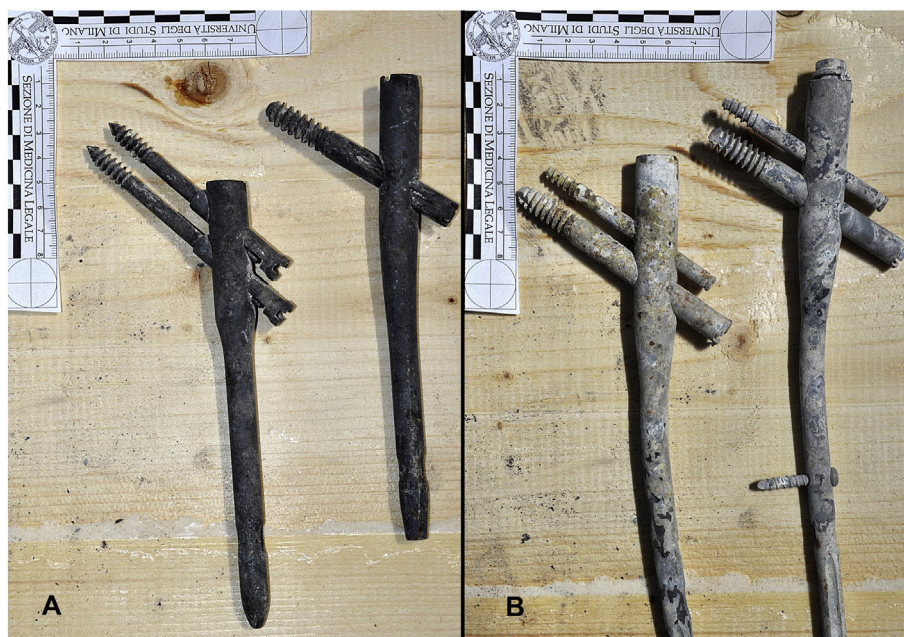
Fig. 1. Four of the 73 endomedullary “gamma-shaped” nails. On the left (A) the dark and heavier metal nails, on the right (B) the bright and lighter ones.
