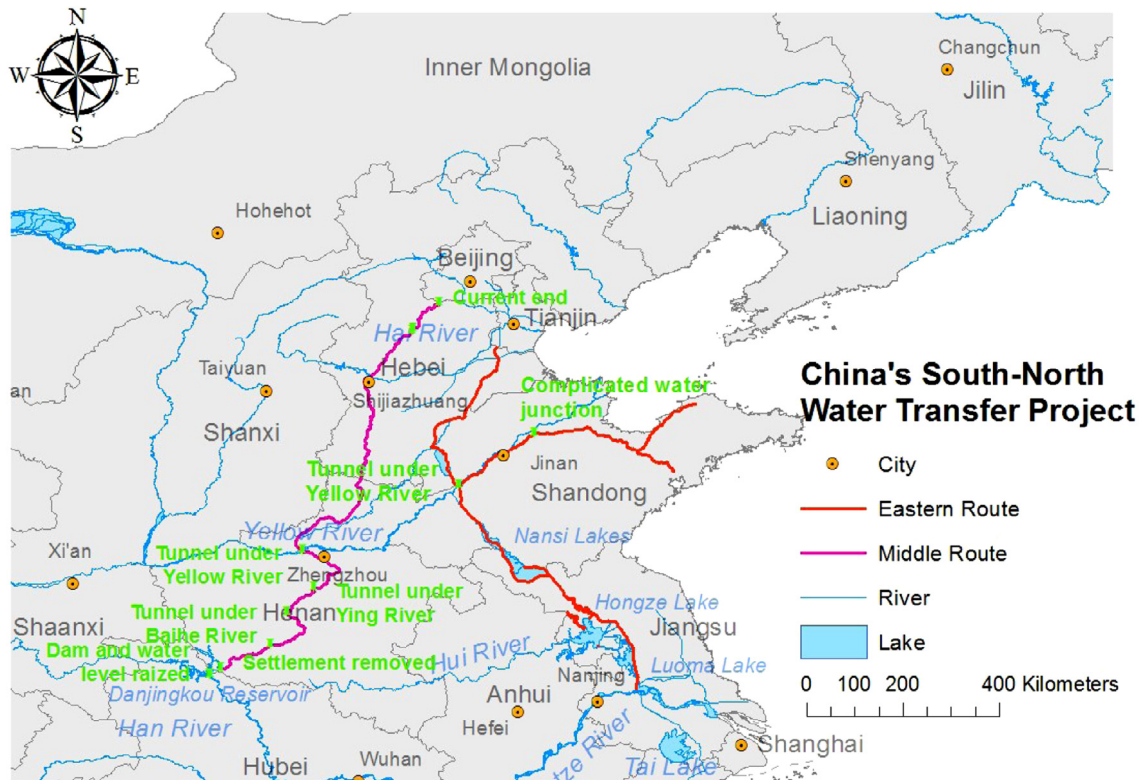
Fig. 1. The Eastern and Middle Routes of China's South-North Water Transfer Project Source: Author's work.
