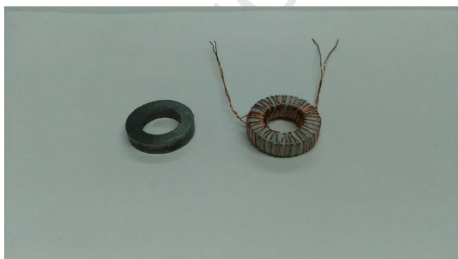
Fig. 1. The toroidal-shaped magnetic cores of the Fe/ZrO 2 SMCs.
