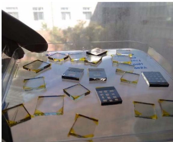
Fig. 1. Prepared devices to study the reproducibility of ZnO/NiO structure on the FTO/glass substrate.
