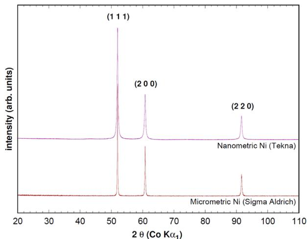
**Fig. 1.** XRD patterns of the two types of powder used, showing the sole presence of Nickel.
