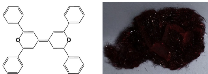
Fig. 1. Left: Chemical structure of 2,2',6,6'-tetraphenyldipyranylidene (DIPO-Ph 4 ). Right: Deep-red shiny crystalline powder of DIPO-Ph 4 after purification by Soxhlet extraction in acetonitrile.
